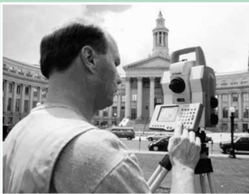
Surveyors today use a total station to measure horizontal and vertical angles automatically.
