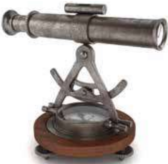
Surveyors once used transits like this one to measure horizontal and vertical angles using a magnifying glass.
