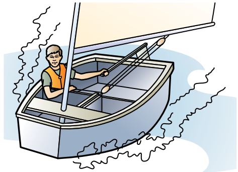
The freestanding mast of an Optimist pram needs no standing rigging.
