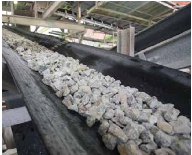
Crushed stone from primary crusher
