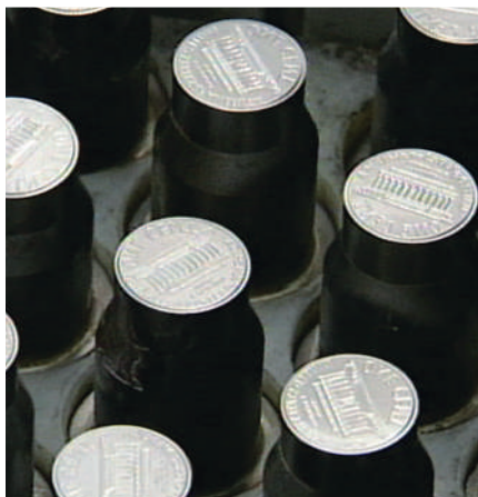
Batches of identical dies can strike many coins at one time.
